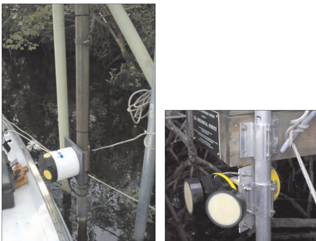
Figure 1-5. Speed-Rail™ mount for sidelooker ADVM. (Left photograph by Marc Zucker, USGS; right photograph by Victor Levesque, USGS.).
