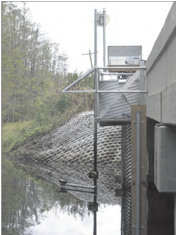
Figure 1-7. Speed-Rail™ mount with sidelooker and uplooker ADVMs mounted to it. (Photograph by Molly S. Wood, USGS.)
