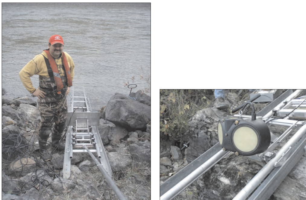
Figure 1-4. Track mount and assembly for a sidelooker ADVM made by Approtek International. (Photograph by Molly S. Wood, USGS.)
