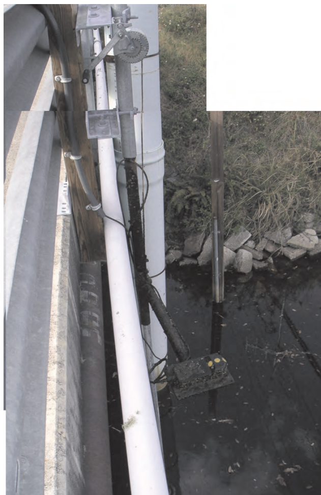
Figure 1-11. ADVM mount with a winch assembly for raising and lowering the ADV. (Photograph by Jeff Banner, Sarasota County, Florida, Used with permission.)
