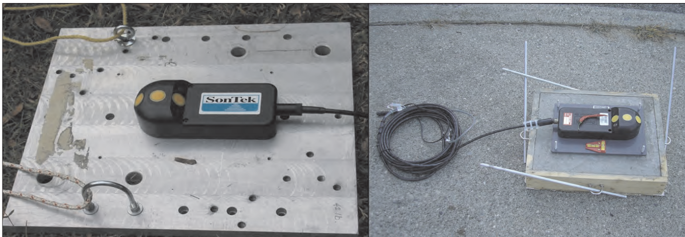
Figure 1-9. Mounting plates for uplooker ADVs. (Left photograph by Molly S. Wood, USGS; right photograph by Marc Blouin, USGS.)
